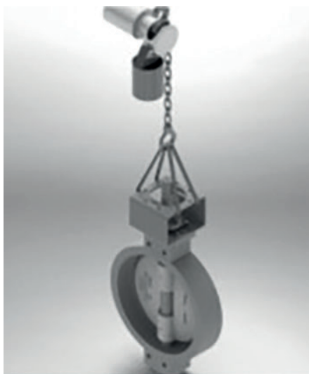
Figure 4-1: Sample lifting points for butterfly valves
