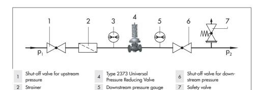
Fig. 6: Installation example for Type 2373 Universal Pressure Reducing Valve
