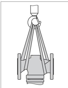
**Fig. 4:** Schematic drawing of lifting points on the regulator
