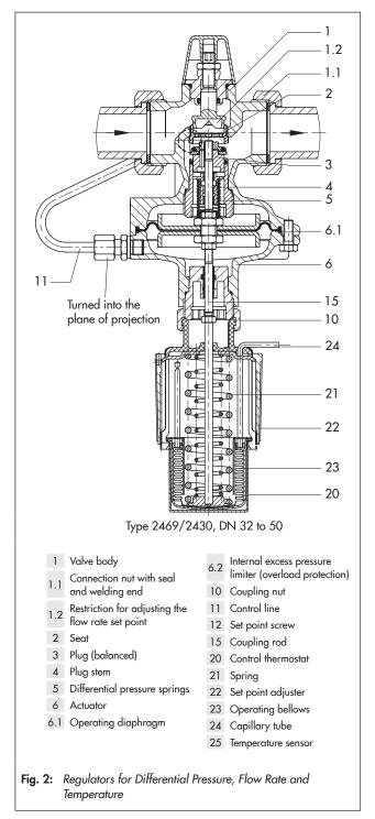
The temperature of the medium creates a pressure in the sensor which is proportional to the measured temperature. This pressure is transferred to the operating bellows (23) and converted into a positioning force. This force moves the valve plug (3) according to the force of the spring (21) and the temperature set point adjustment.
