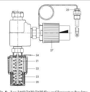
Fig. 4: Type 2469/2430/2439 Flow and Temperature Regulator and Safety Temperature Limiter
