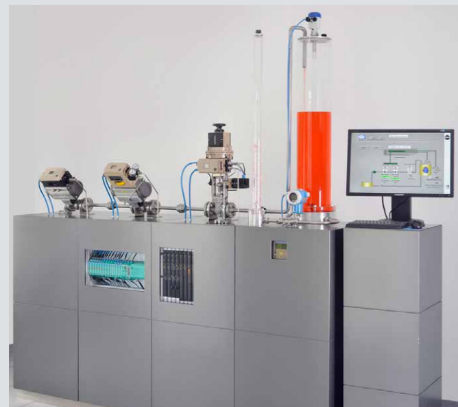
Fig. 1 · Demonstration model of a safety-instrumented system at SAMSON
